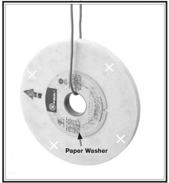
Figure 20. Ring test setup and test locations.
